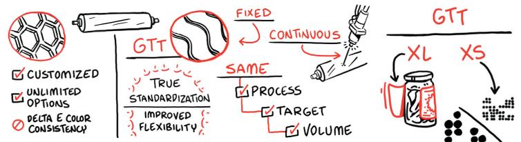
From GTT XL for high opacity white printing to GTT XS for superfine and high-definition process work, GTT 2.0 can replace your entire stockpile of conventional anilox with a handful of GTT sizes, and significantly reduce the number of ink recipes required to achieve pantone colors.
