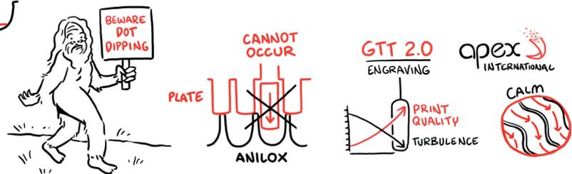
Thanks to the wave-based flow of ink on the anilox surface, liquid up-lift created by angular acceleration is now a thing of the past. The new, improved engraving ensures up to 50 % reduction of cell wall surface area across the anilox, at the same time decreasing the required channel depth by an average of 25%.
