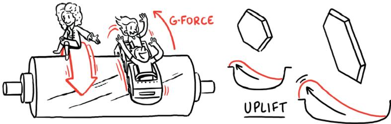
Let's take a closer look at the surface of an anilox and apply Newton's second law of rotation to a conventional anilox cell. As the anilox rotates, the ink inside each cell is pushed backwards colliding with the back-cell wall. This results in the ink rising from the cells creating a bubble effect on the surface of the anilox.
