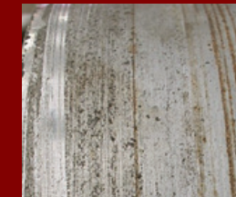
Look familiar? Typical flaking and corrosion on chrome-plated glue roll; scoring on doctor roll.
